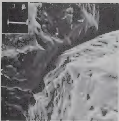
7.8a Interpenetrative grain contact.
